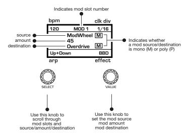
Using the Mod Matrix to assign the Mod Wheel
