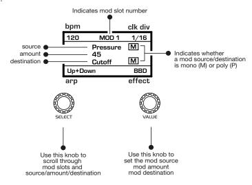
Using the Mod Matrix to assign the pressure (aftertouch)
