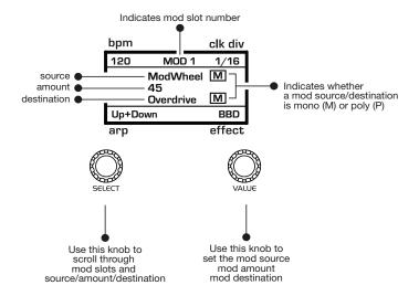
You already understand and apply the concept of modulation whenever you use the filter envelope to control the filter's cutoff frequency. In this case, the modulation *source* is the filter envelope (or more precisely, any of its controls, such as attack, decay, sustain, or release). The modulation *destination* is the filter's CUTOFF frequency. The modulation *amount* is set with the Filter Envelope's AMOUNT knob.
